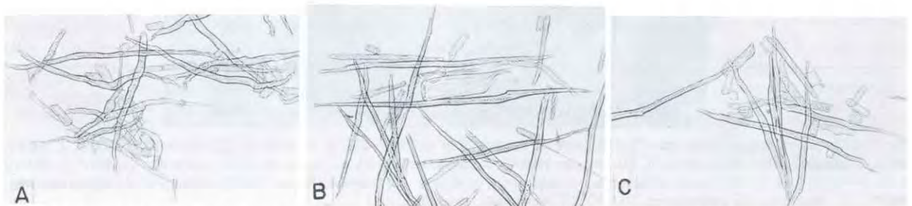
Fig. 5. Macerated material of A. tumor wood (briarwood), B. stem wood, and C. root wood of Erica arborea (35 \times ).
